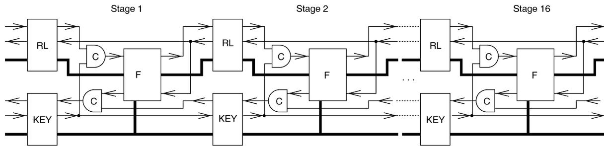
Fig. 3. Fine-Grain pipelined asynchronous DES.
