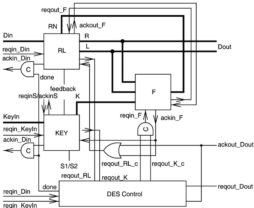
Fig. 2. Area-Optimized asynchronous DES.
