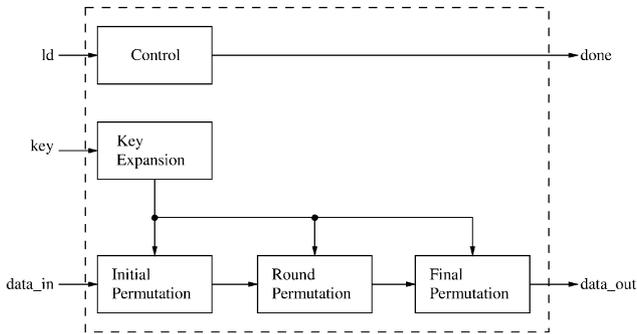
Fig. 5. Encryption AES module.
