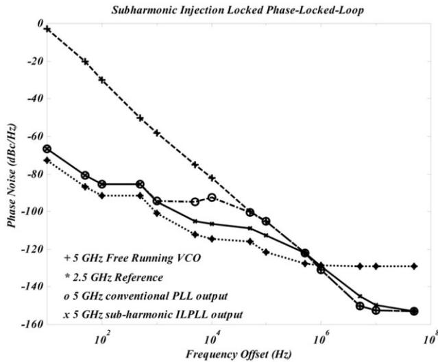
**Figure 3** Calculated results for the output phase noise of the proposed S-ILPLL and a conventional PLL with the same components
