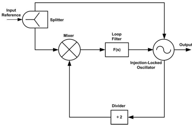
Figure 1 Subharmonic injection-locked phase-locked-loop
