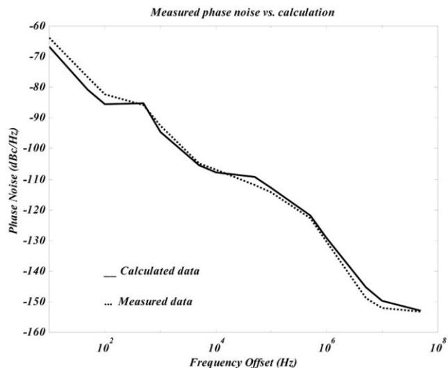
Figure 7 Measured data and calculated results for phase noise
