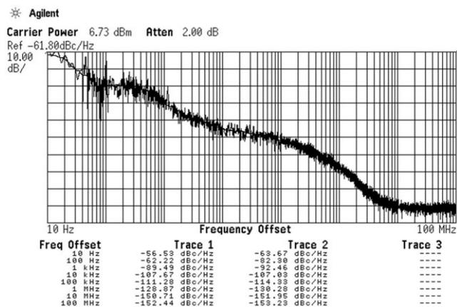
Figure 5 Phase noise measurement of the S-ILPLL
