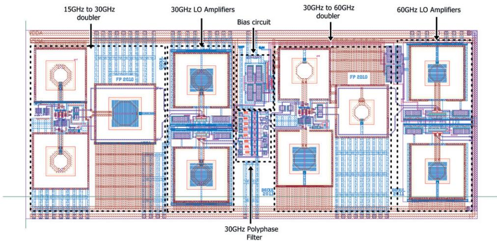
Figure 19. The layout of the frequency quadrupler.
