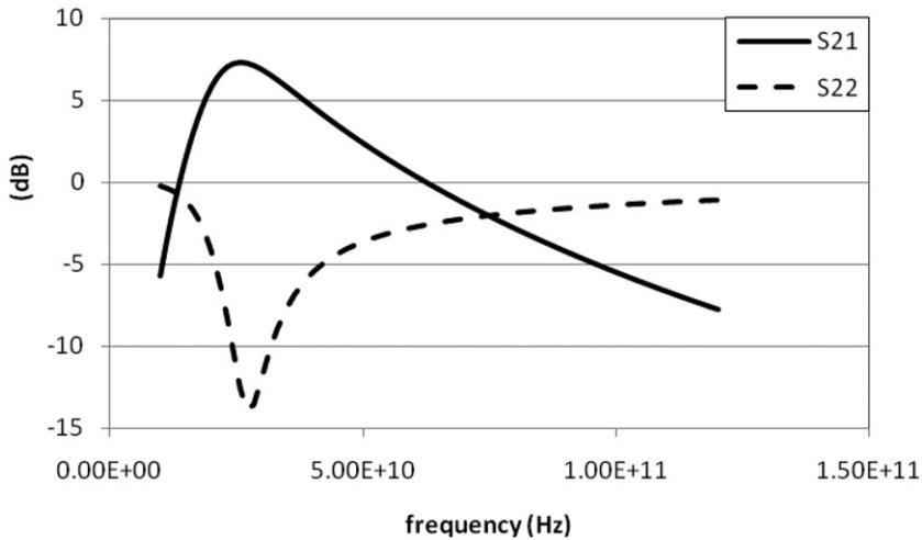
Figure 15. Simulation results of the LO amplifier at 30 GHz.
