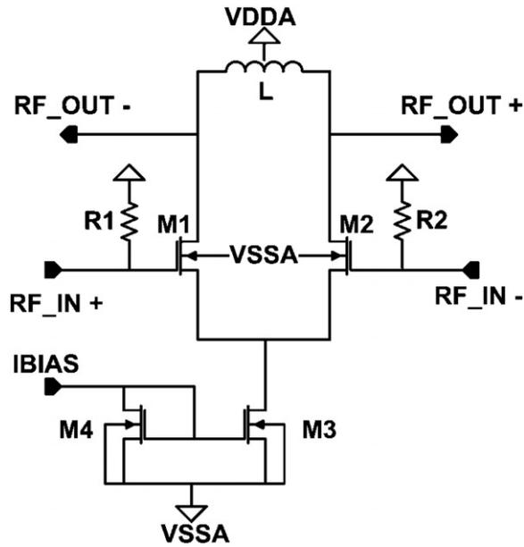
Figure 14. The schematic of the LO amplifier.
