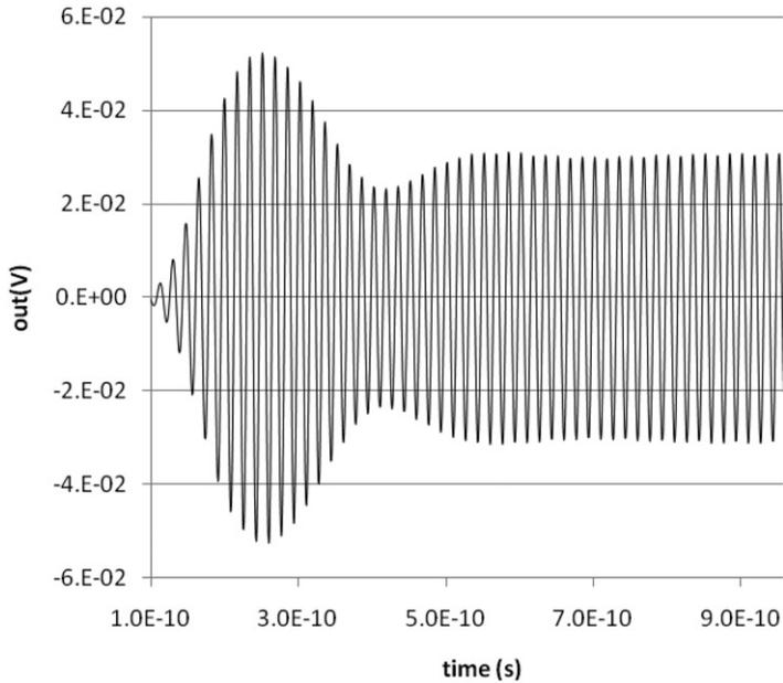
Figure 20. The 60 GHz output of the frequency quadrupler.
