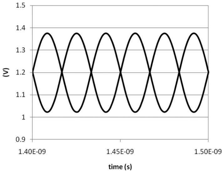
Figure 9. Input signals of the polyphase filter.
