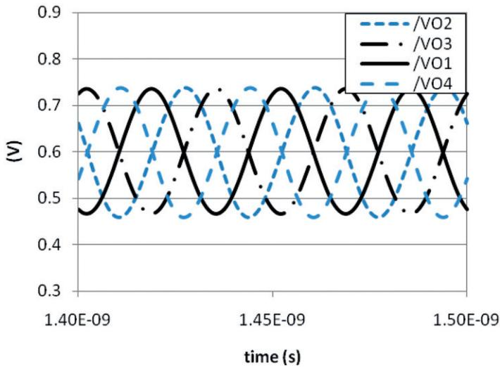
Figure 12. Output signals of the active polyphase filter.
