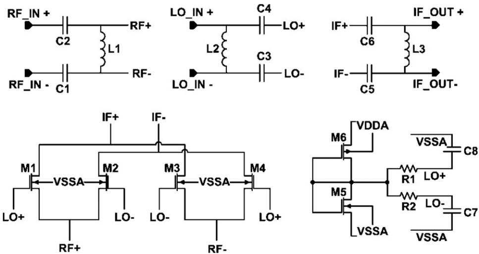
Figure 3. The complete schematic of the frequency doubler.
