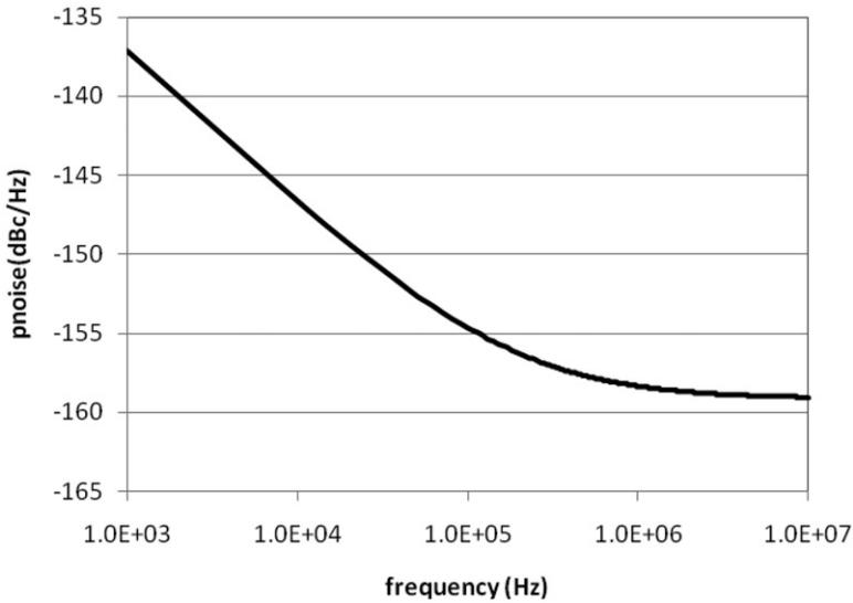
Figure 16. Phase noise simulation results of the LO amplifier at 30 GHz.
