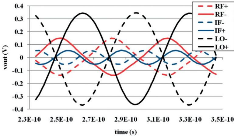
Figure 4. 30 GHz doubler transient simulation results.
