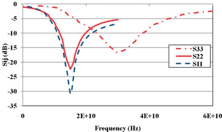
Figure 5. 30 GHz doubler input/output matching.
