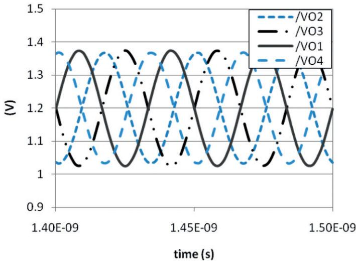
Figure 10. Output signals of the passive polyphase filter.
