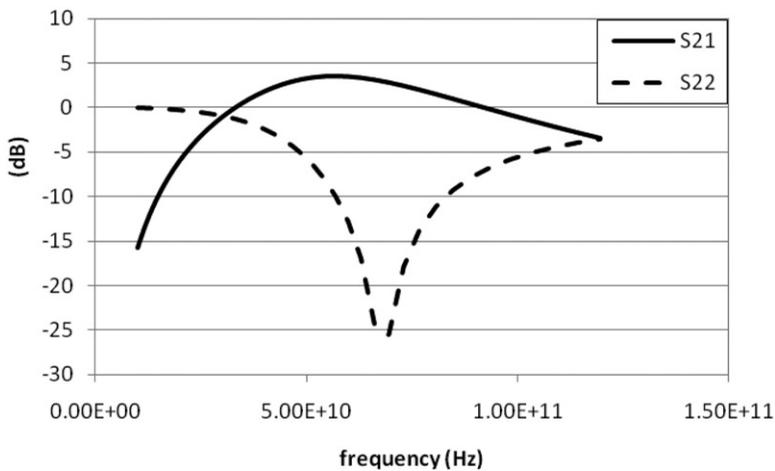
Figure 17. Simulation results of the LO amplifier at 60 GHz.
