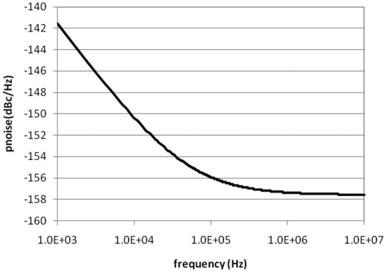
Figure 18. Phase noise simulation results of the LO amplifier at 30 GHz.
