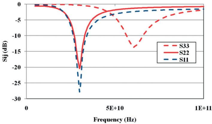
Figure 7. 60 GHz doubler input/output matching.
