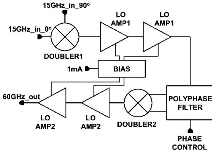
Figure 1. The full quadrupler topology.
